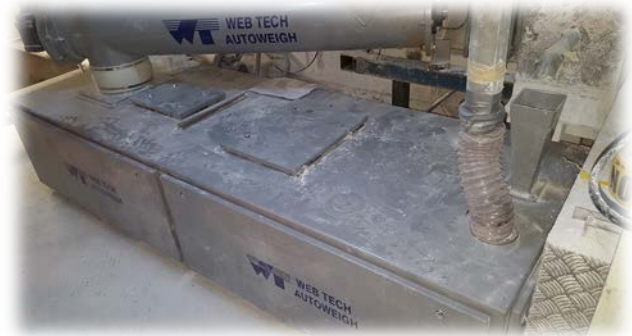
Screw pre-feed is suitable for applications where the material must be contained
